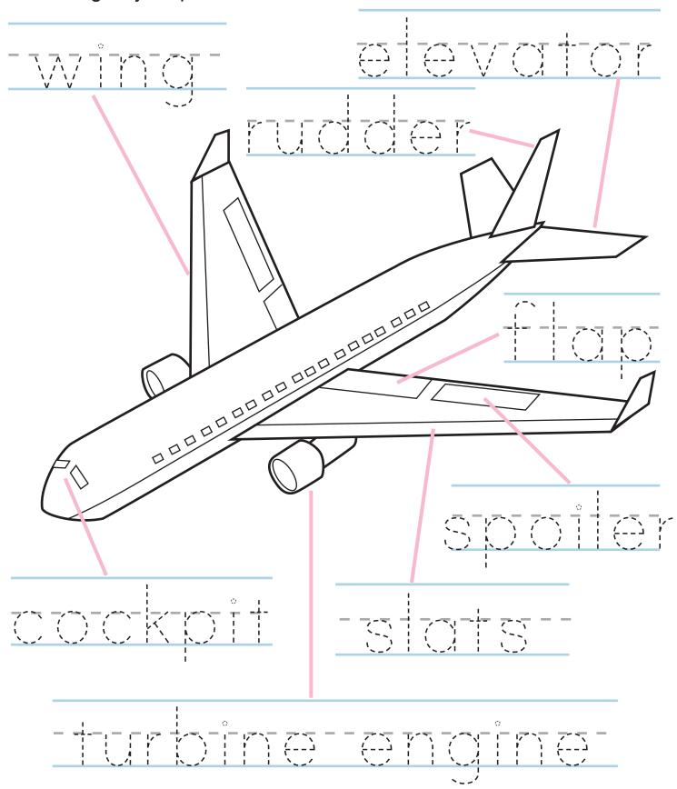
The parts of the plane all work in different ways. Check out these parts that help the plane take off, fly, and land. Read aloud to your child to explain important parts of the plane, and sound out any of the words that are new or difficult for him.
